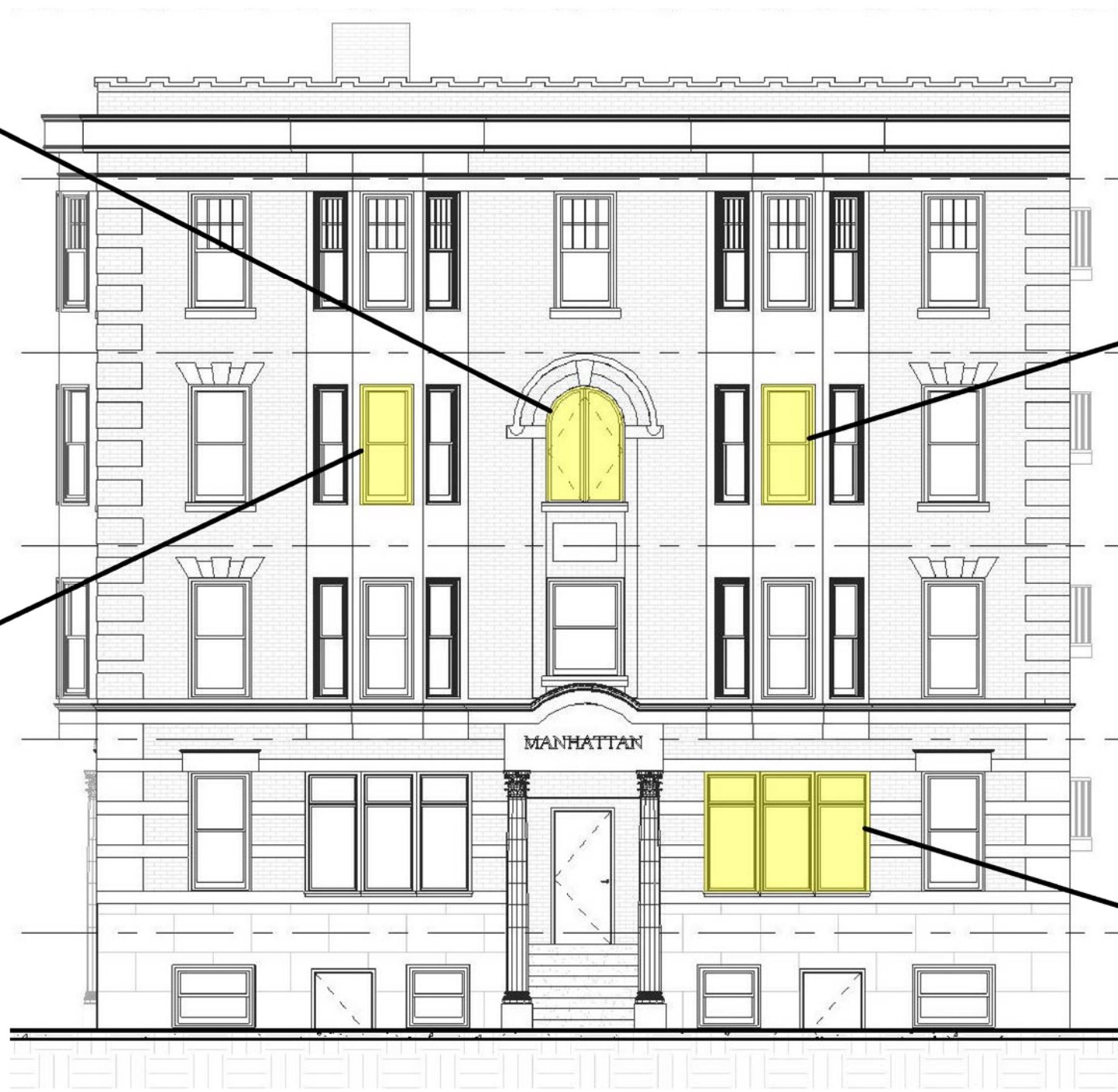
1 MANHATTAN - SECOND AVE FACADE - WINDOW MAPPING 1/4" = 1'-0"
