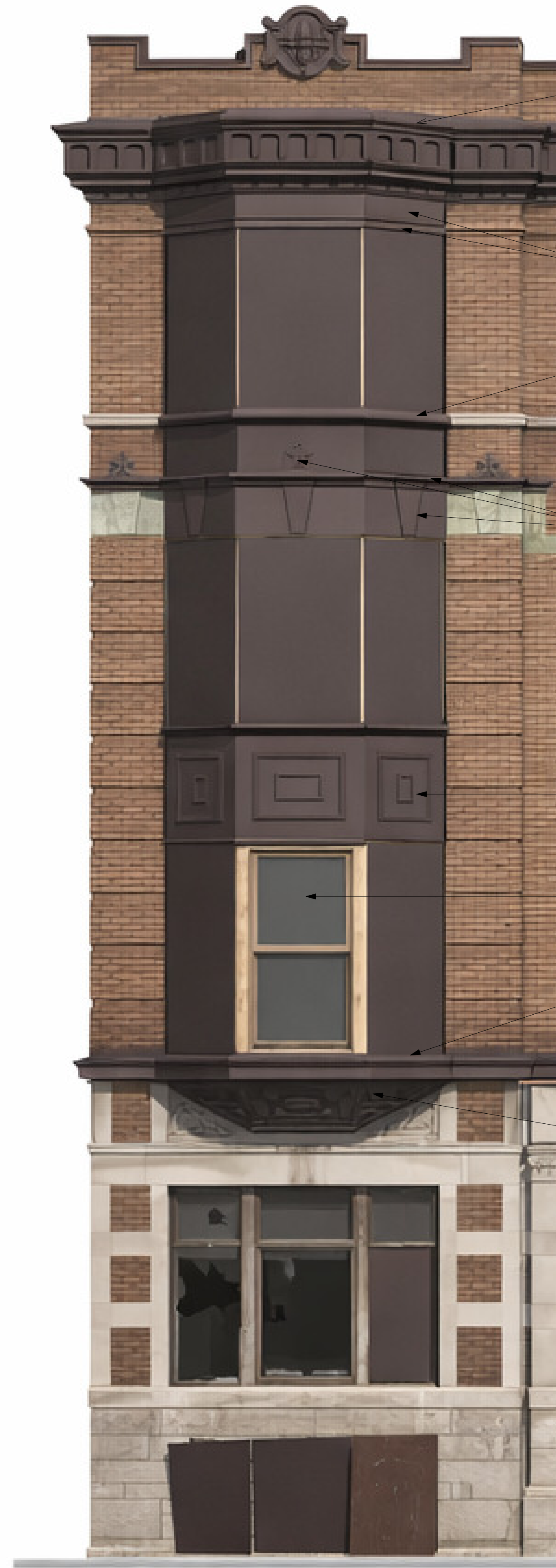
1 A-0.3.2.1 3/8" = 1'-0" TYPICAL BAY ELEVATION - ALTADENA
