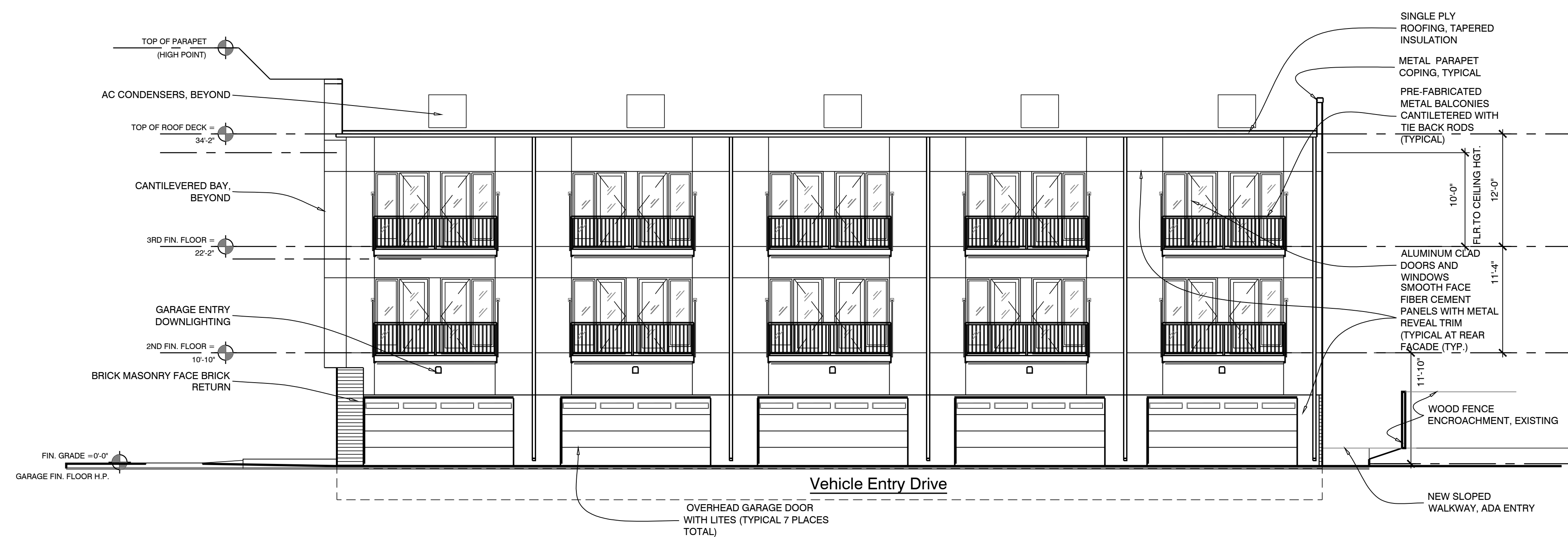
Rear Building 1- North Elevation
