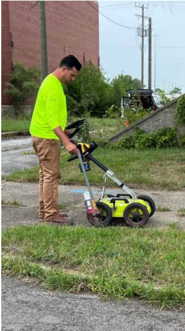
Figure 10 Ryan from GPRS operating the GPR unit
