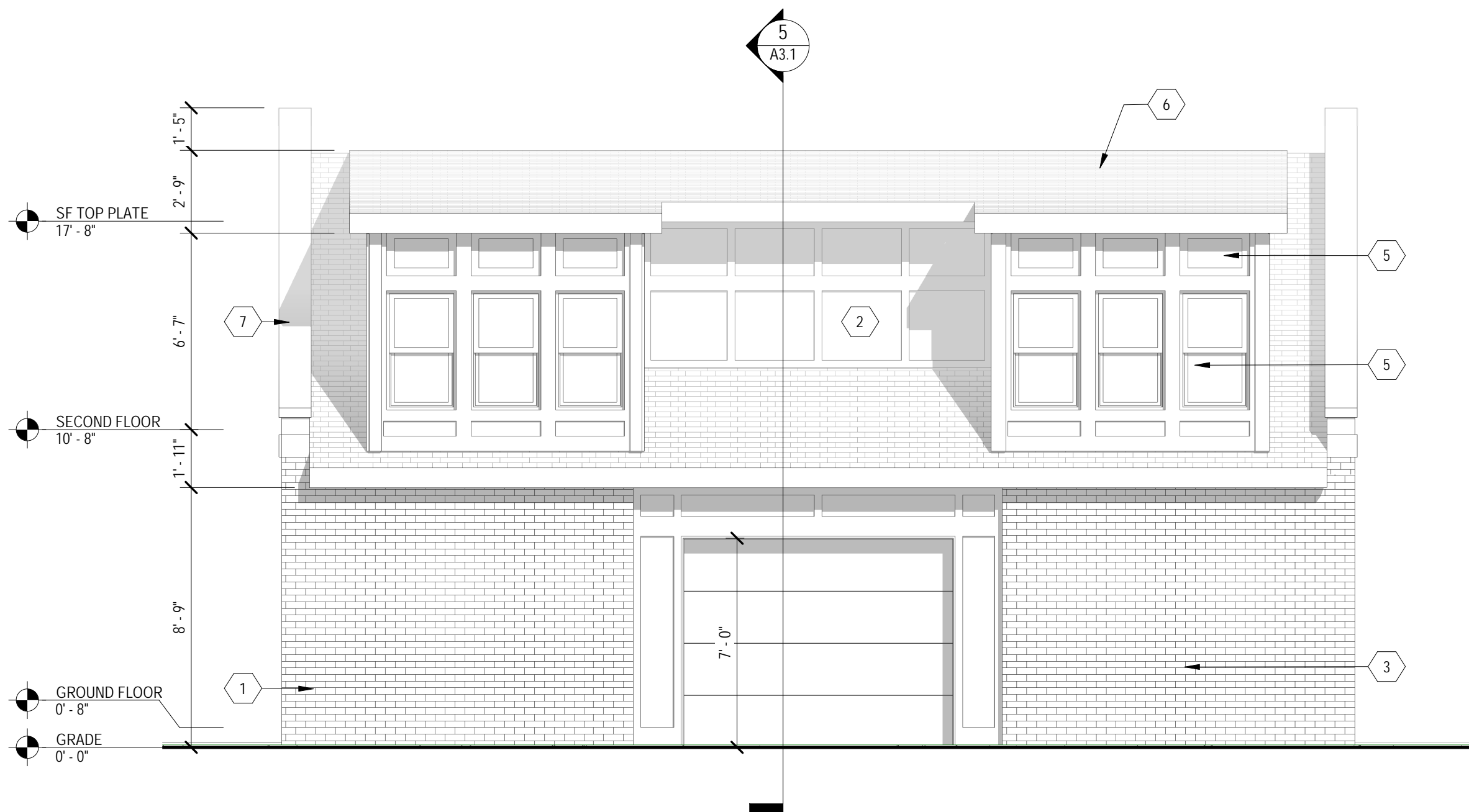
3 NORTH (ALLEY) ELEVATION SCALE: 1/4" = 1'-0"
