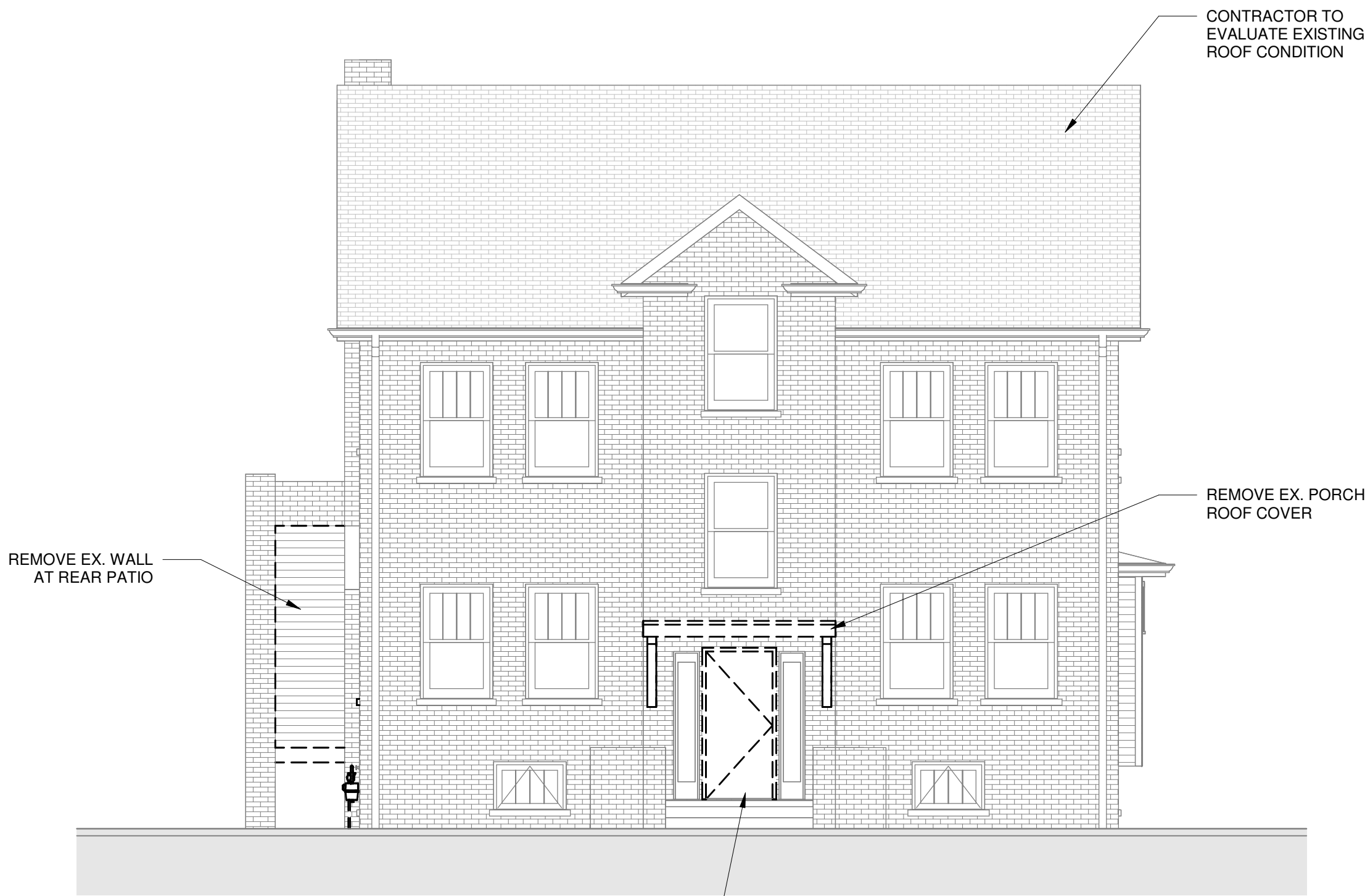
1 WEST ELEVATION - DEMO 3/16" = 1'-0"
