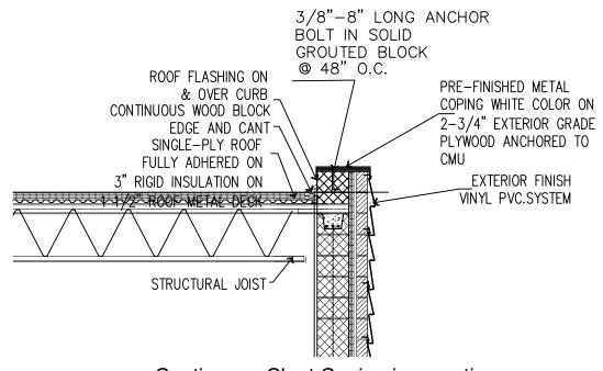
Continuous Cleat Coping is a continuous perimeter roof edge system designed to cap parapet walls.
