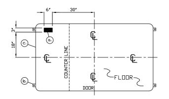
NOTE: PROVIDE 120/240V. 10-3 WIRE SERVICE WITH GROUND. SERVICE ENTRANCE/ANCHOR BOLT LAYOUT
