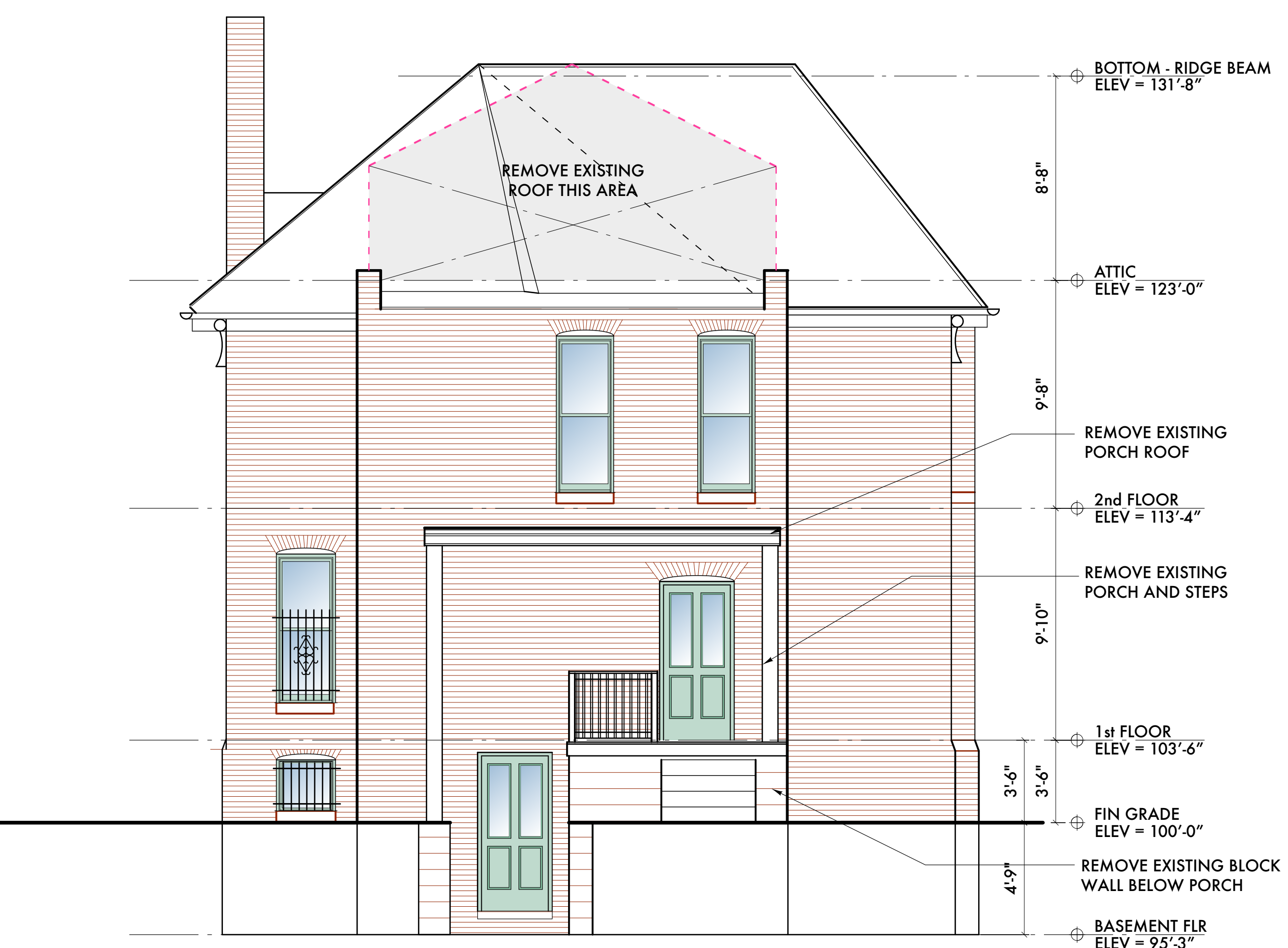
C SOUTH (ALLEY) ELEVATION 1/4" = 1'-0"
