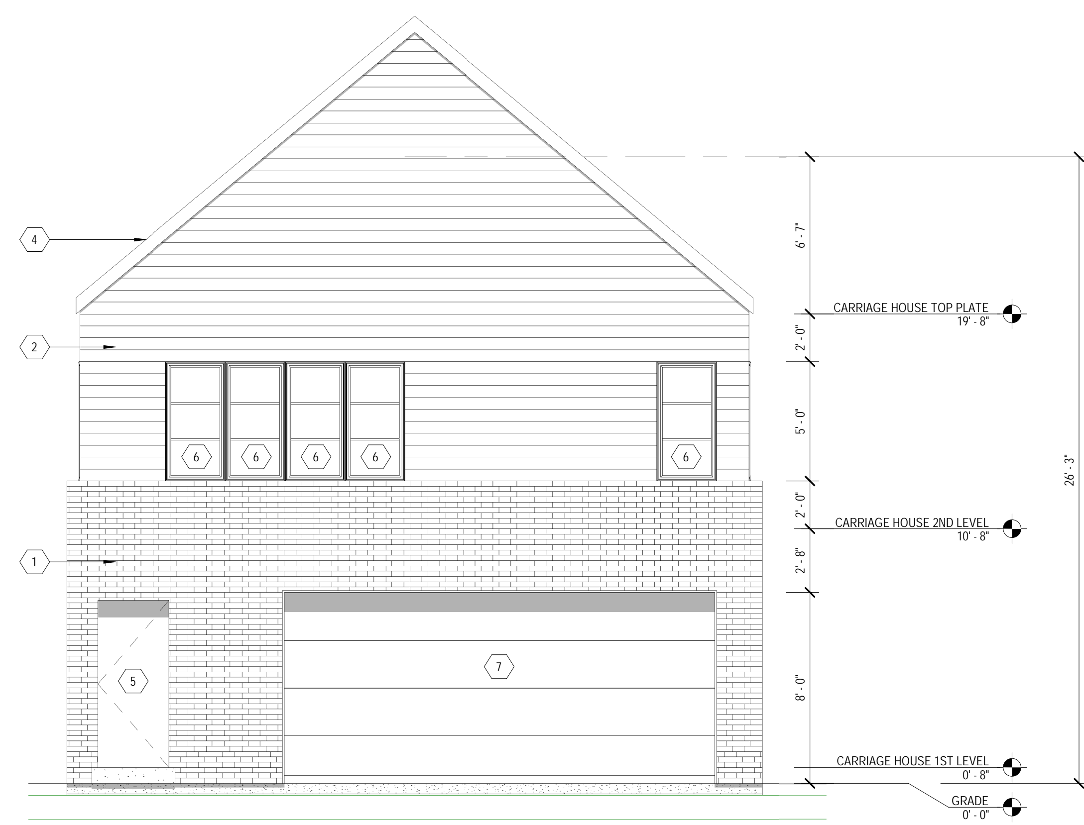
3 EAST ELEVATION-CARRIAGE HOUSE SCALE: 1/4" = 1'-0"
