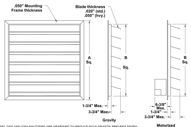
THE MODEL GSS AND GSH SHUTTERS ARE DESIGNED TO REDUCE BACK DRAFTS; PREVENT ENTRY OF SOME FOREIGN MATERIAL AND PESTS, SUCH AS BIRDS; AND LIMIT THE AMOUNT OF RAIN THAT ENTERS THE BUILDING. THESE SHUTTERS ARE INTENDED TO BE WEATHER-RESISTANT, BUT ARE NOT WEATHER-PROOF FOR EXTREME CONDITIONS.
