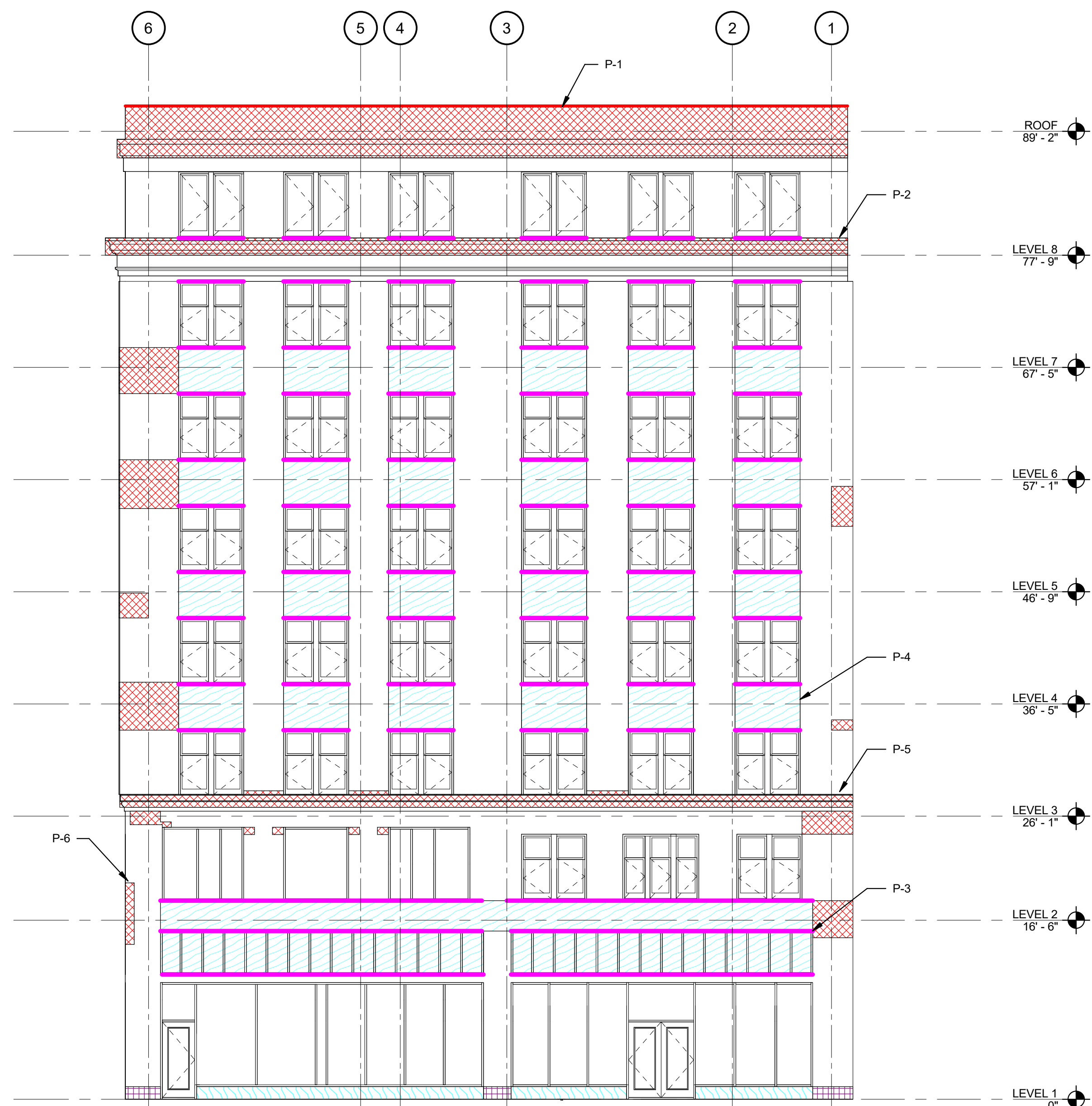
PRELIMINARY WEST ELEVATION REPAIRS SCALE: 1/8" = 1'-0"
