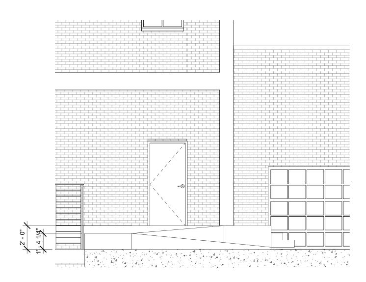
12 STAIR B ADA ACCESS RAMP - EAST ELEVATION SCALE: 1/4" = 1'-0"
