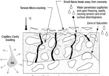
Pore and Capillary swelling causes tension cracking.
