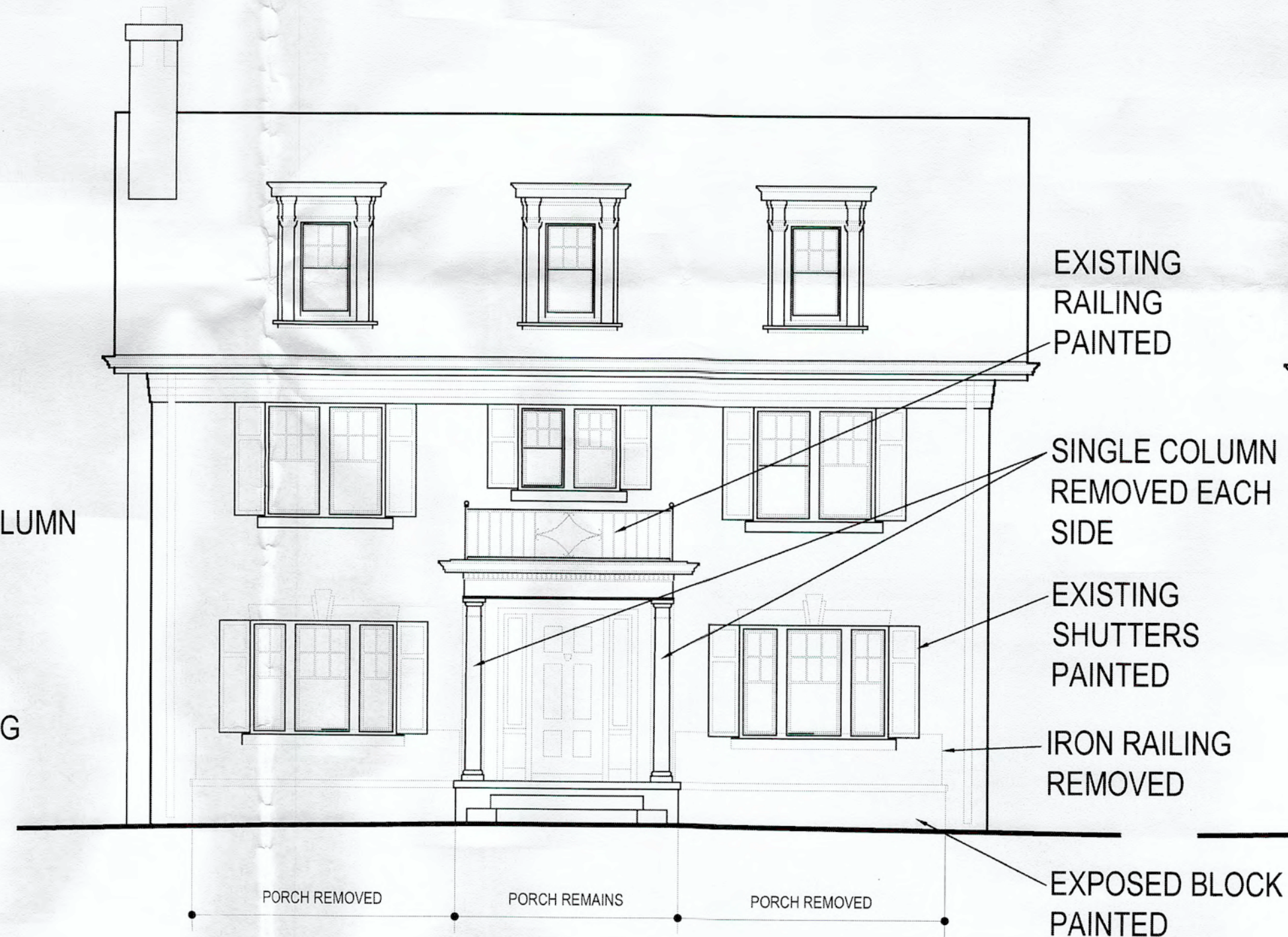
2 NORTH ELEVATION - 2017 ALTERATIONS A1.1 3/16"=1'-0" 0 6'-0"
