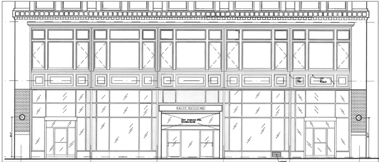
Elevation drawing of new aluminum storefront and canopy, approved by HDC in 2004.
