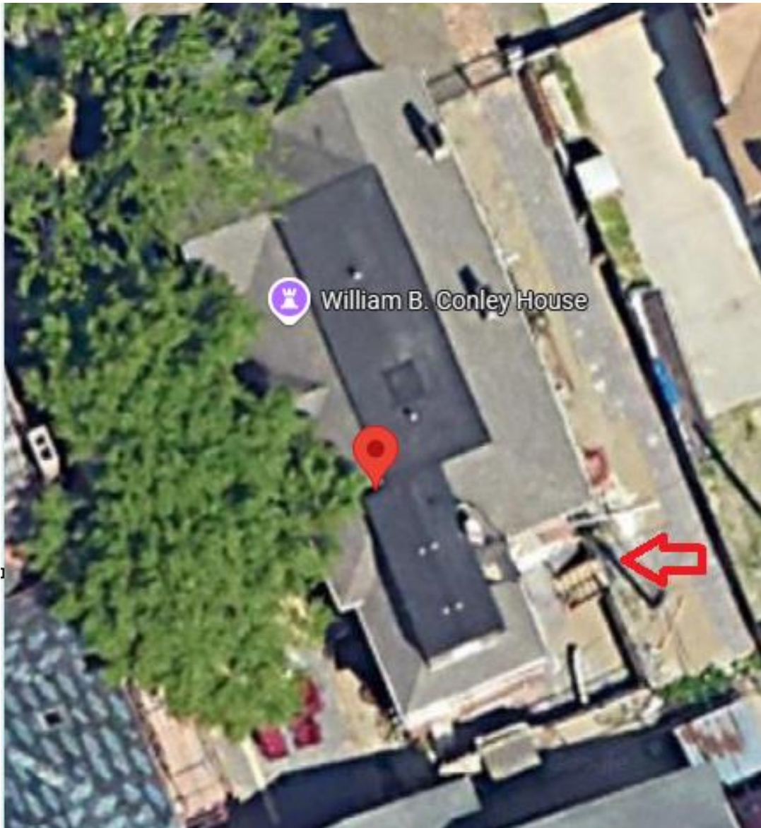
Photo 4. 691 W Canfield, existing conditions, Google map, 2025, exposed trench behind the house is visible. Beginning at the rear of the house on the east side (at the southeast corner) and continuing across the entire rear of the house, the exposed trench is visible. Steps leading down into the trench are visible in this image near the house's southeast corner, at red arrow.
