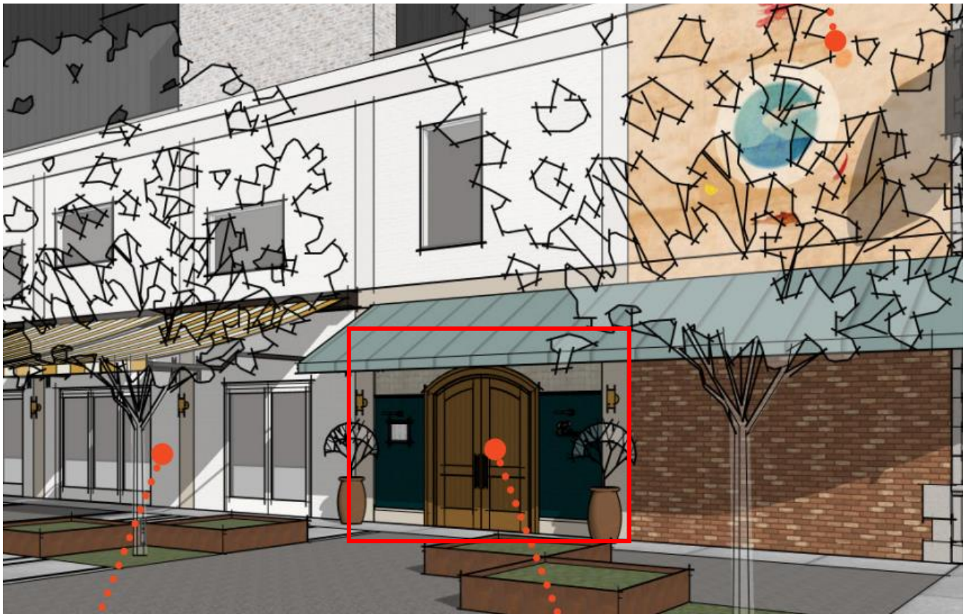
Proposed new wood entry doors. New tile and limestone trim will be installed within this bay
