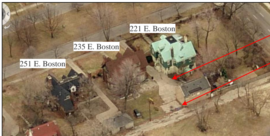
This aerial view shows the footprint of the shared driveway between 221 and 235 E. Boston, as well as the footprint of the concrete pad that supported the original garage for 235 E. Boston. Due to the narrow driveways for the three houses visible in this photo, coupled with the width of the existing historic-age 2 – 3 car garages, concrete aprons spanning the width of the garages were poured. ConnectExplorer, March 26, 2006.
