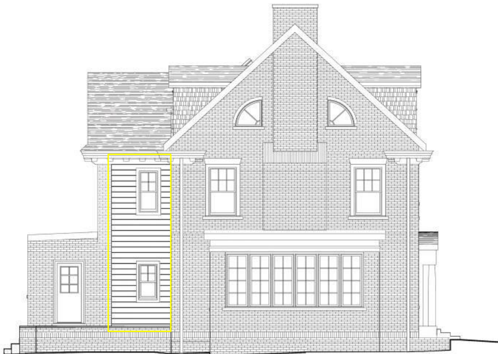
Above elevation drawings, submitted by applicant showing proposed condition/proposed new lapped wood siding at rear wall (outlined in yellow)
