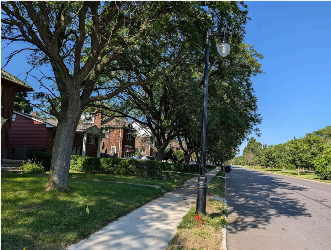
View of an existing fiberglass pole in the Oakman Boulevard Historic District. Staff photo, August 7, 2024.
