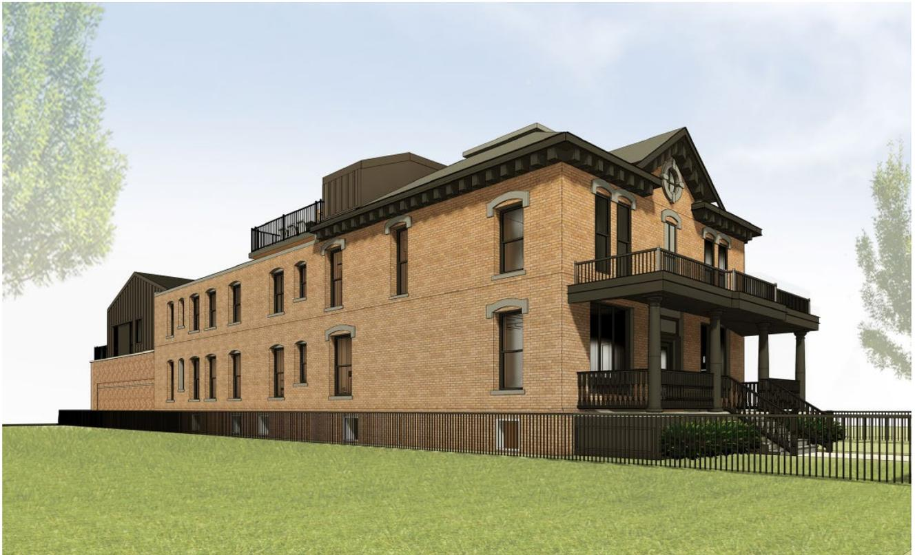
*Rendering of view from Edmund Place, east side of building, showing rooftop deck alterations and new addition visible at far left.*
