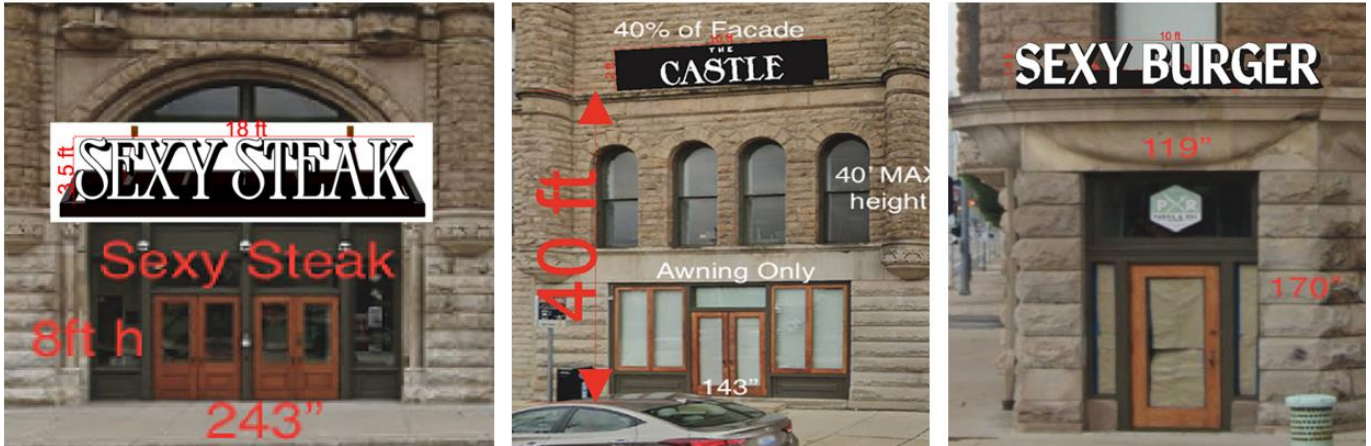
Proposed signs, left to right: 18’x3.5’ sign on Grand River (southwest) façade; 10’x2’ sign on Adams (northwest) façade; 10’x1.5’ sign at east corner entrance. Note that the Grand River sign projects forward on an aluminum awning.
