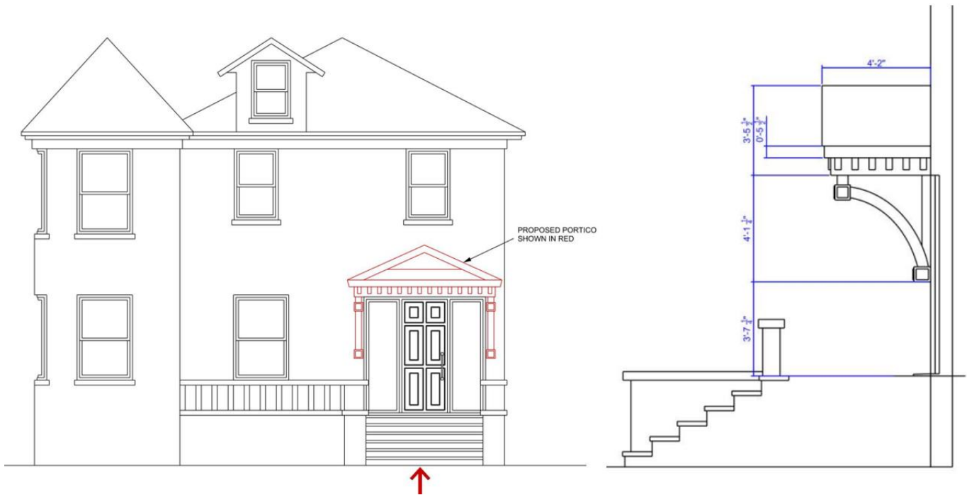
Elevation (left) and section (right) of proposed pediment. Images from submitted drawings, cropped by staff.
