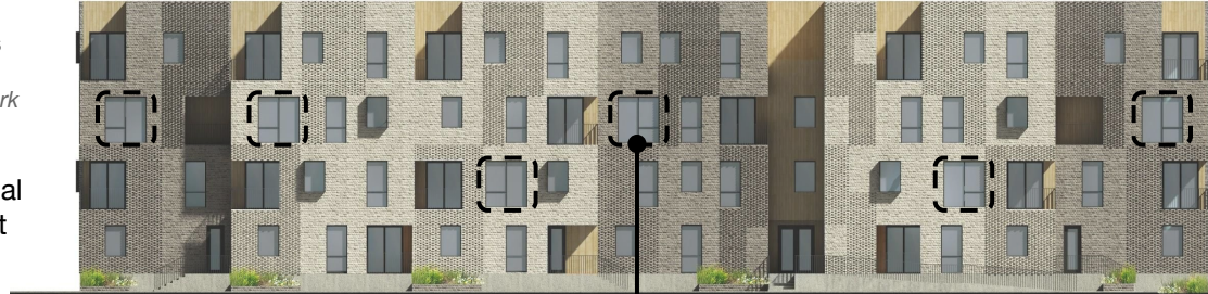
— — Newly added combined windows
