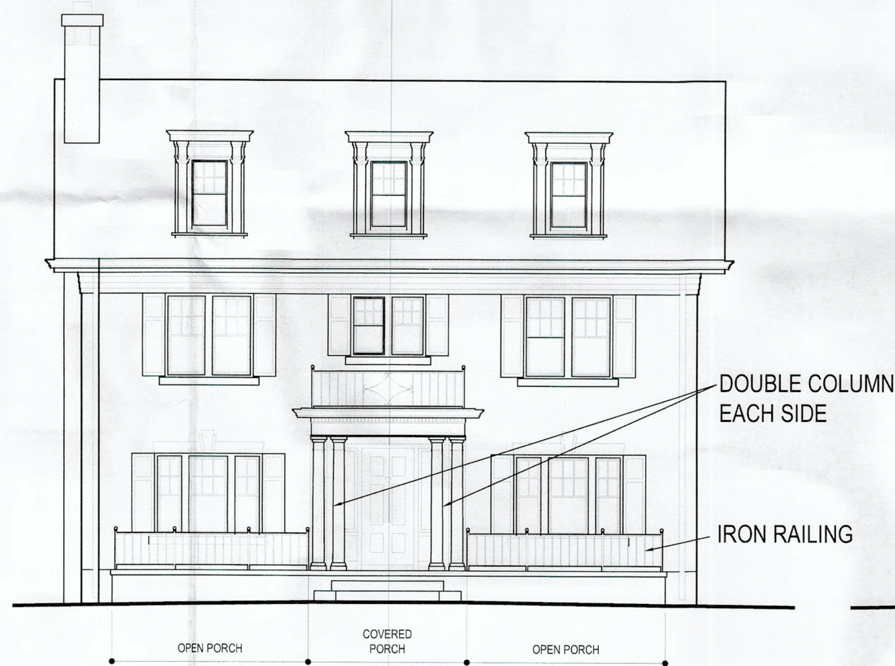
3 NORTH ELEVATION - ORIGINAL CONDITION A1.1 3/16"=1'-0" 0 6'-0"
