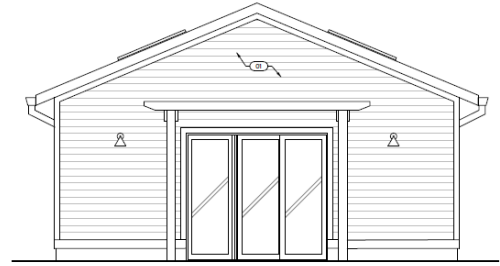
2 WEST ELEVATION (SIDE YARD) SCALE: 3/8"=1'-0"
