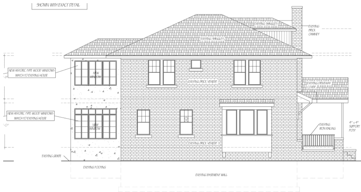
PROPOSED LEFT SIDE ELEVATION SCALE 1/4" = 1'-0"
