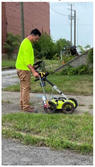
Figure 10 Ryan from GPRS operating the GPR unit
