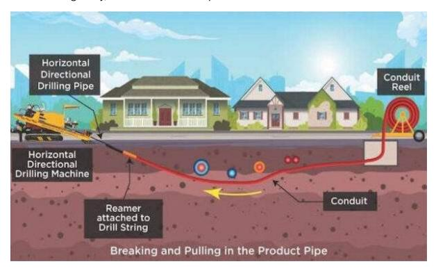
Figure 5: general HDD diagram
