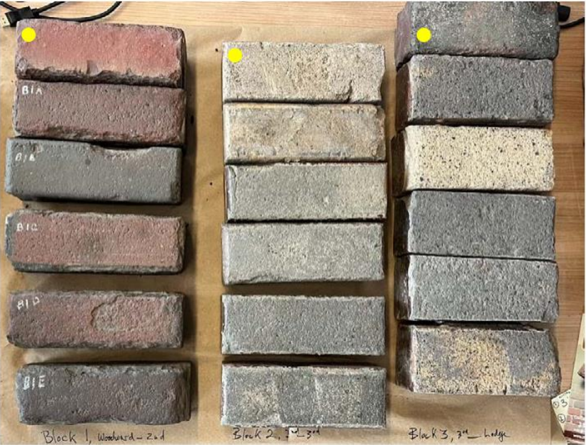
Block 1: 9" x 3" x 4" Block 2: 9" x 3 1/4" x 4" Block 3: 8.5" x 3 5/8" x 4"
