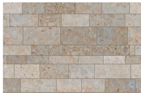
LIMESTONE IN A FINE ASHLAR MASONRY PATTERN - GROUND FLR. VENEER AT COURTYARD FACADE
