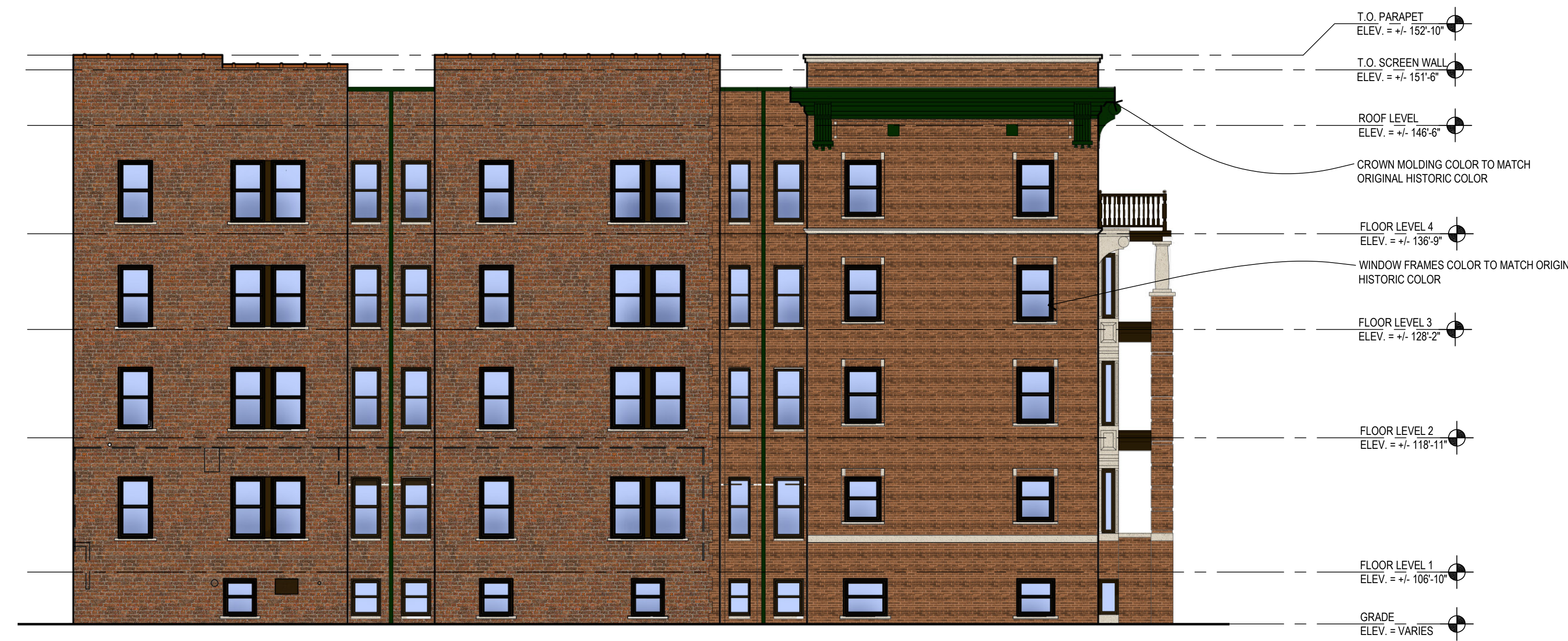
2 6A401.1 2467 CASS SOUTH EXTERIOR ELEVATION 1/8" = 1'-0"
