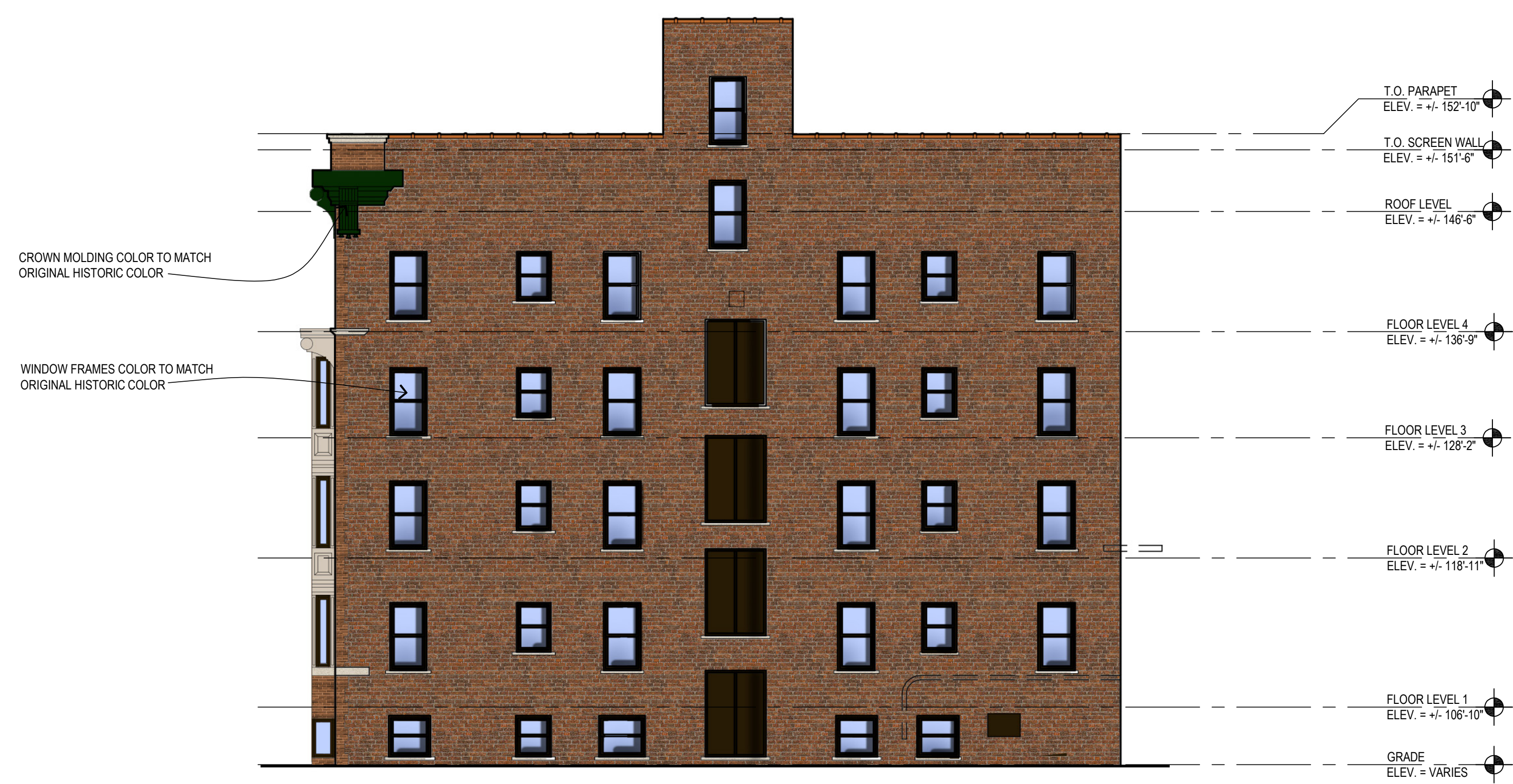
4 6A401.1 2467 CASS WEST EXTERIOR ELEVATION 1/8" = 1'-0"
