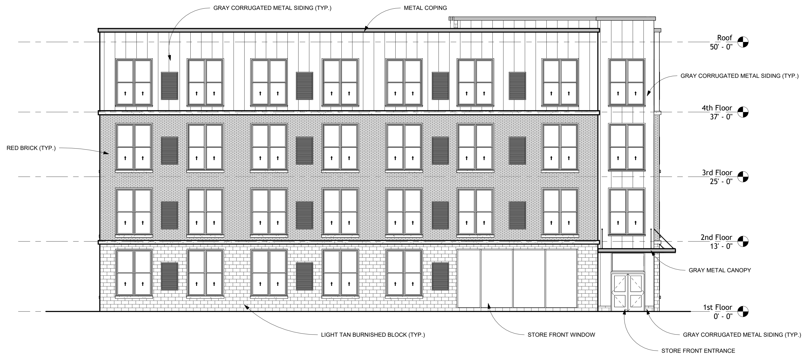
① West Architectural Building Elevation 1/8" = 1'-0"
