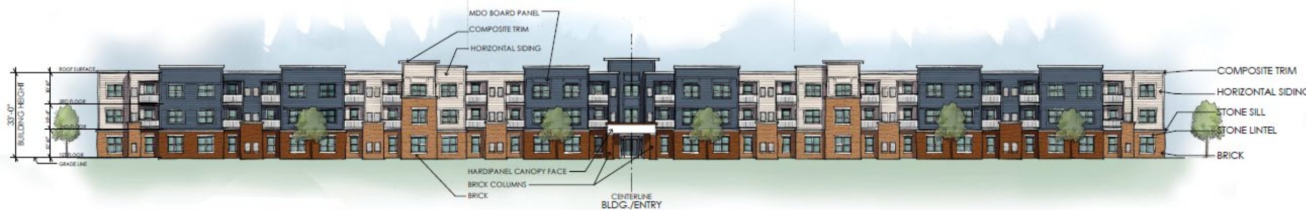
FRONT (STREET) ELEVATION APARTMENT BUILDING
