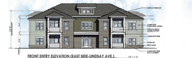
FRONT ENTRY ELEVATION (EAST SIDE-LINDSAY AVE.) 1-BEDROOM UNIT BUILDING - REAR ELEVATION SIM. 1/8" = 1'-0"
