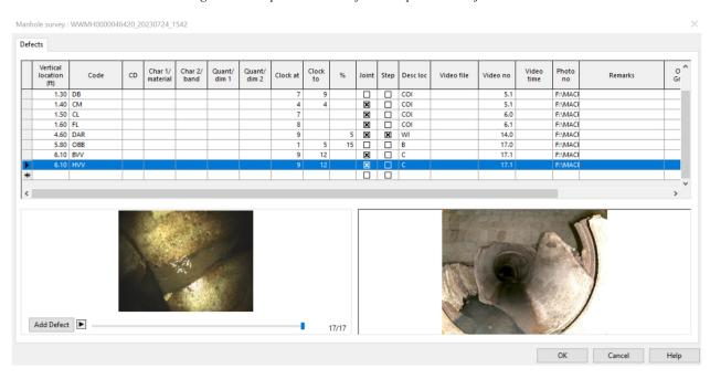
Figure 4 – Sample Manhole Defect from a Manhole in the Project Area
