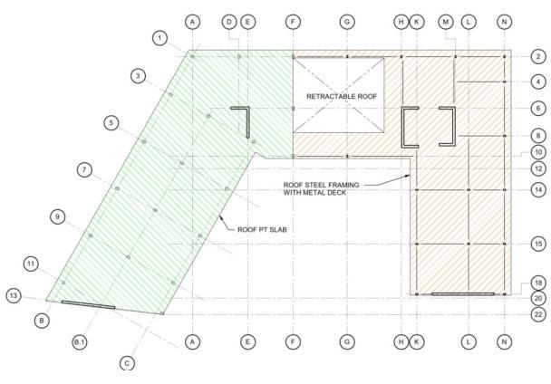
Figure 4: Roof Framing
