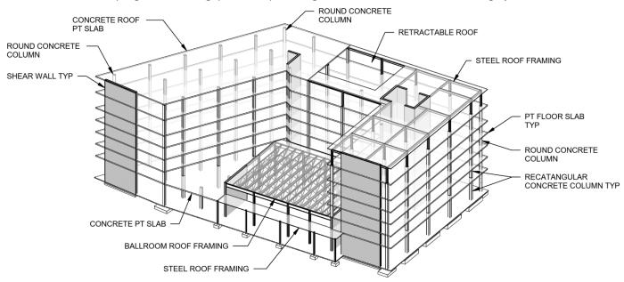
FIGURE 1: CONCRETE BUILDING SYSTEM
