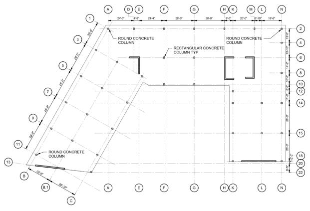
FIGURE 3: CONCRETE COLUMN LOCATIONS
