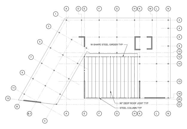
FIGURE 8: BALLROOM ROOF FRAMING
