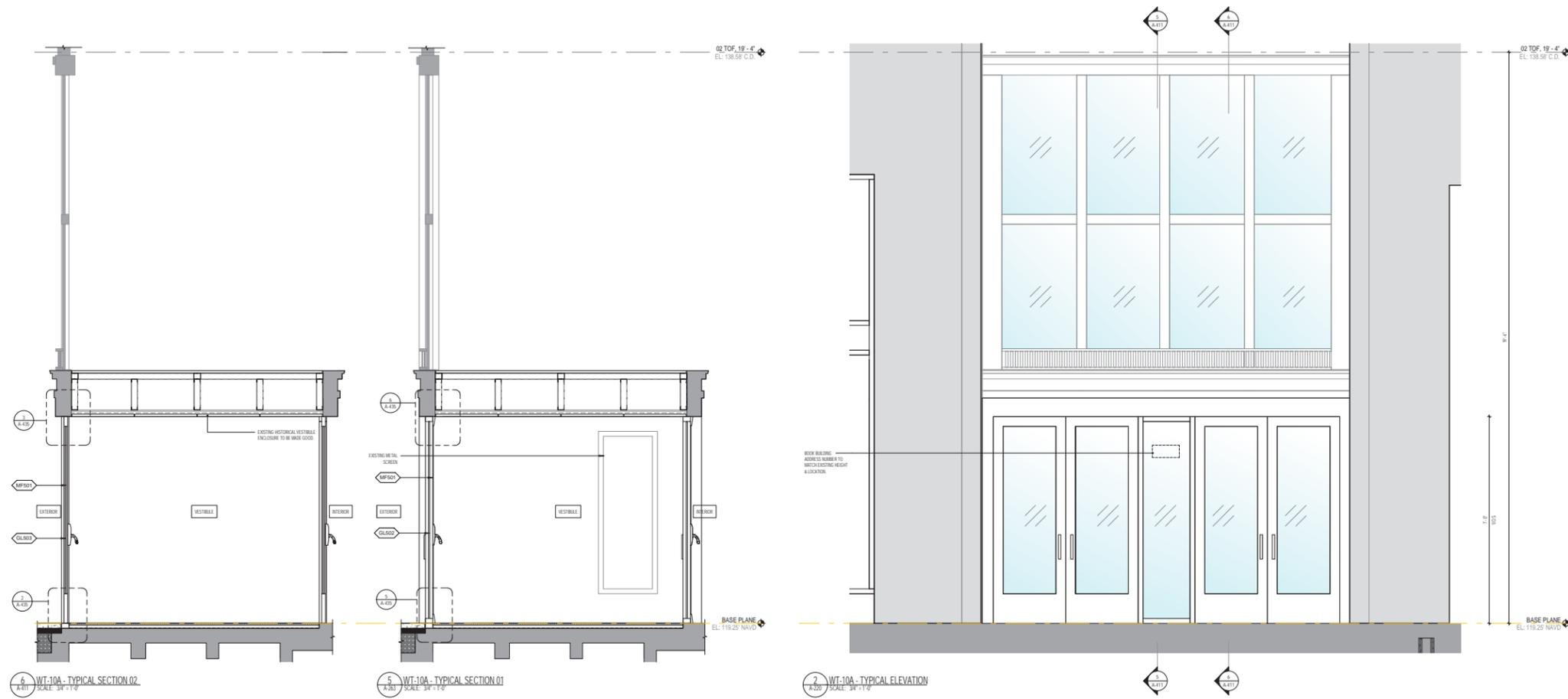
**MF501** EXTERIOR STEEL FRAMING. PAINT COLOR/SIZE/FINISH TO MATCH EXISTING.
