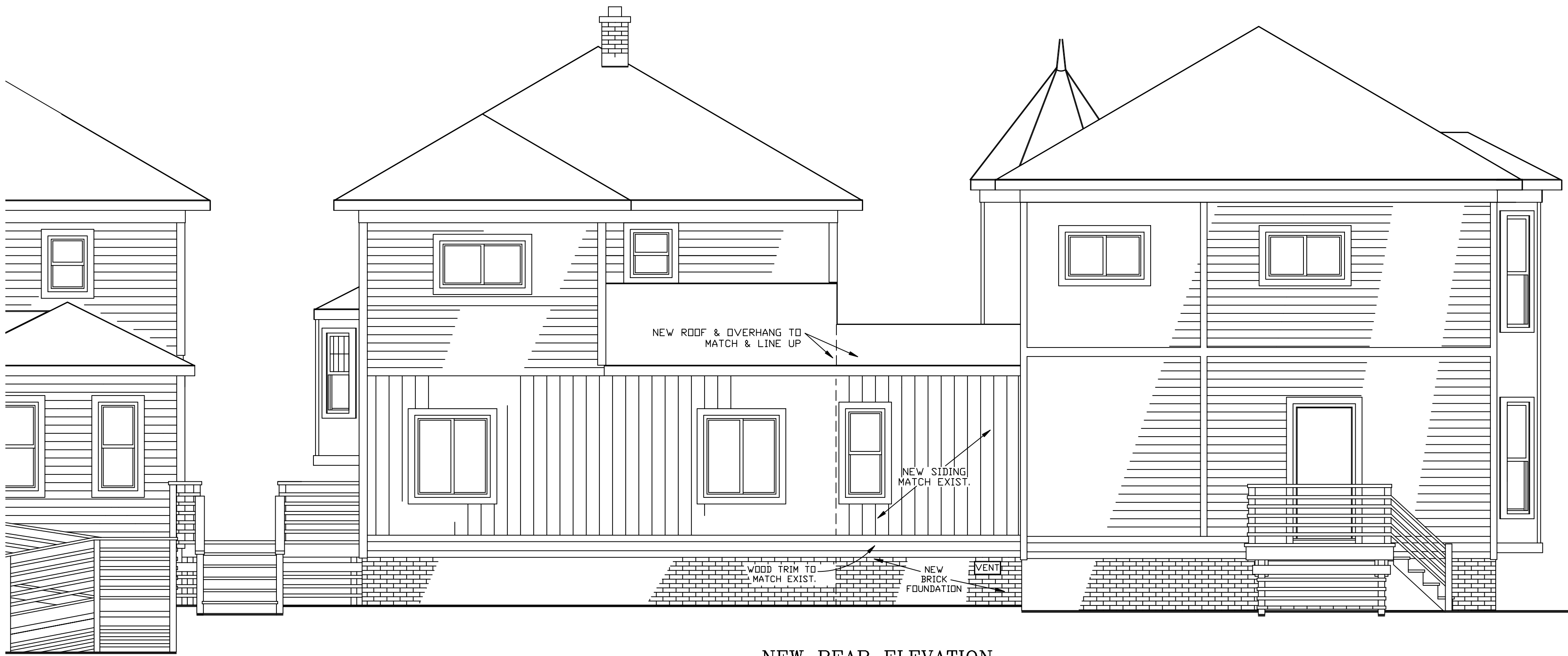
NEW REAR ELEVATION WITHOUT WOOD FENCE SCALE - 1/4" = 1'-0"
