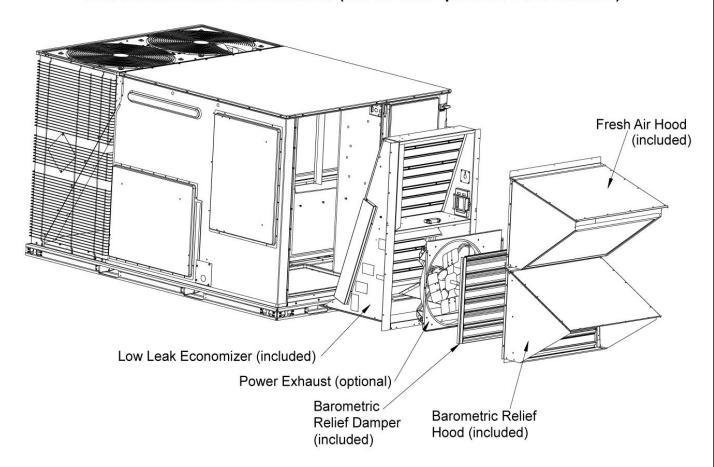
Low leak economizers are capable achieving low leakage rates of 3 cfm/sq. ft at 1" of static pressure, meeting or exceeding the following standards:
