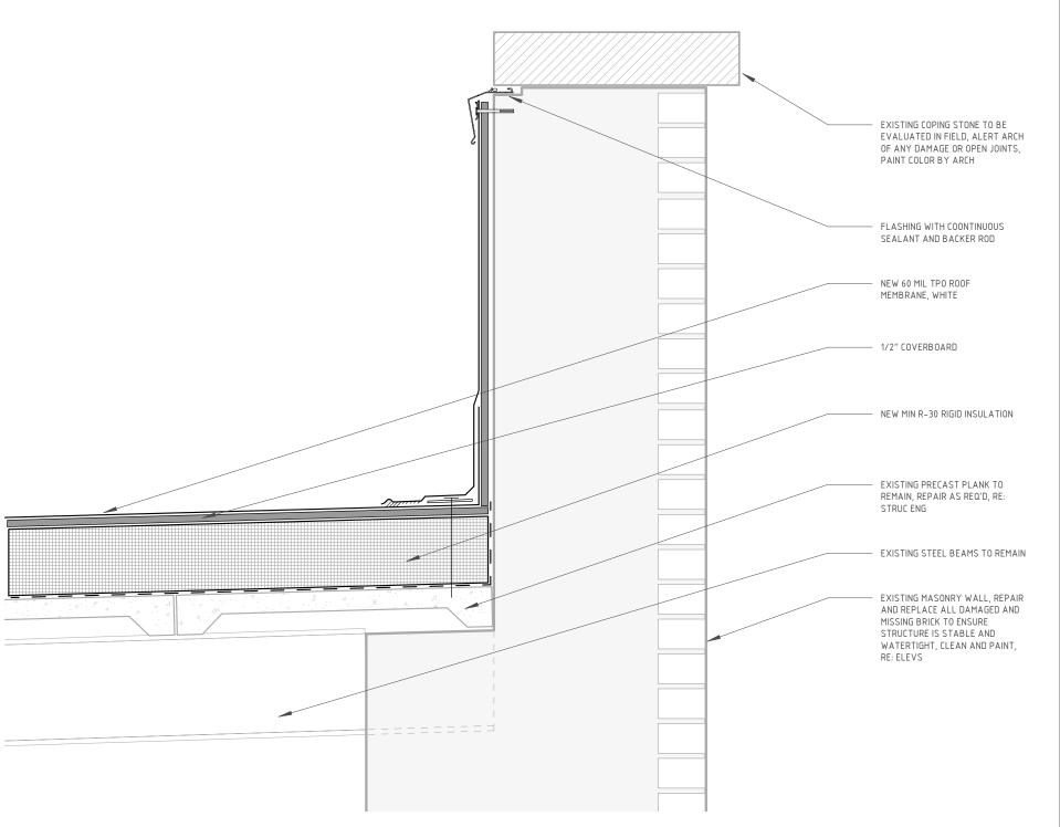
DETAIL 2863 TYP PARAPET AND NEW ROOF
