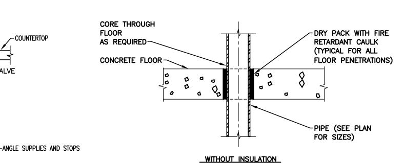
PIPE SLEEVE THROUGH FLOOR DETAIL
