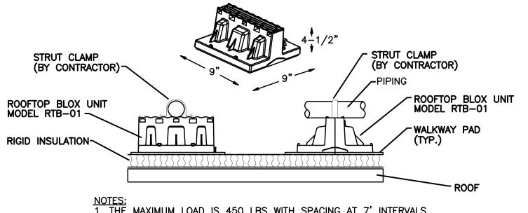
MAXIMUM LOAD IS 450 LBS WITH SPACING AT 7' INTERVALS. 2. LOADS ABOVE 250 LBS REQUIRE THE USE OF STRUT (TO DISTRIBUTE THE WEIGHT LOAD). 2. THE LOAD MUST BE CENTERED ON THE ROOFTOP BLOX UNIT. 3. THE PIPING SHALL BE ATTACHED USING STANDARD STRUT CLAMPS.
