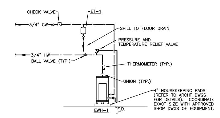
ELECTRIC WATER HEATER DIAGRAM, DWH-1
