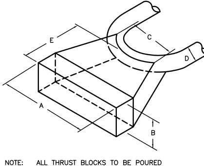
AGAINST UNDISTURBED EARTH WITH MINIMUM 3000 P.S.I. STRENGTH CONCRETE @ 28 DAYS
