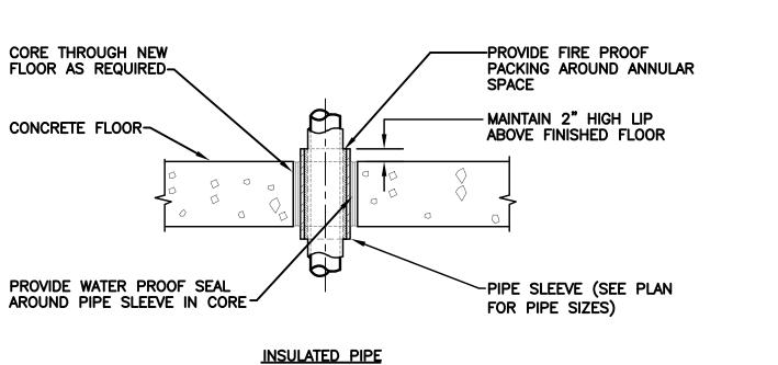
PIPE SLEEVE THROUGH FLOOR DETAIL
