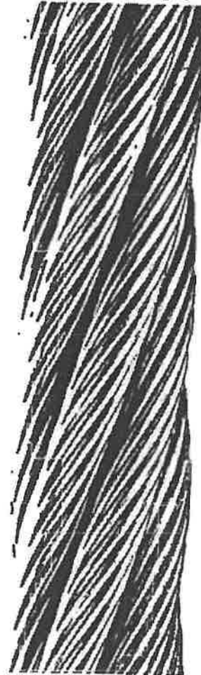
6 x 21 filler wire Type U rope with IWRC and lang lay
