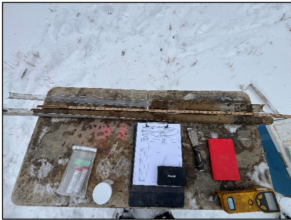
Photo 7: Viewing 5532 SB03 soil recovery, facing northeast
