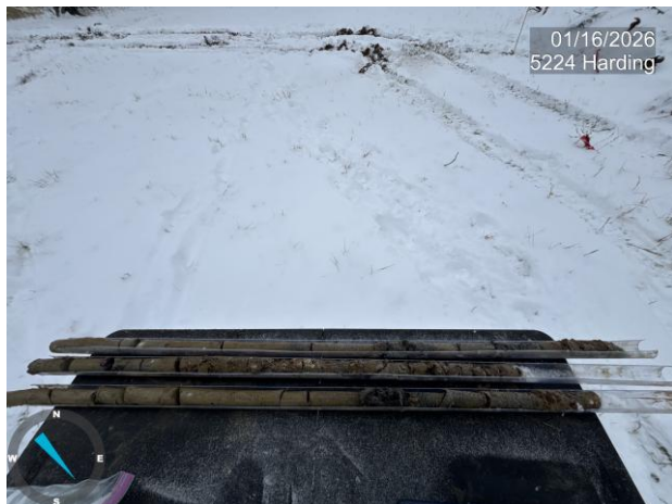
Photo 7: Viewing the soil recovery from 5224 SB-01, SB-02, and SB-03 (back to front), facing southeast.
