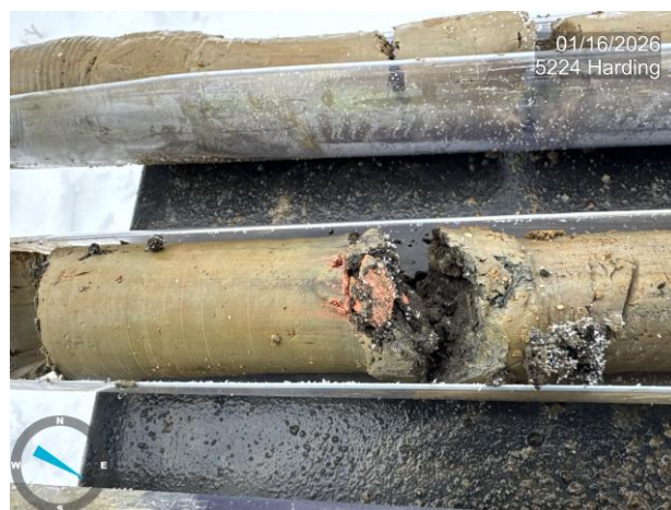
Photo 6: Viewing debris in 5224 SB-02 at 5' bgs, facing southeast.
