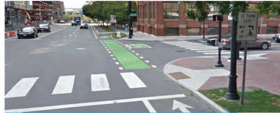
Two stage turn queue boxes are used to provide cyclists with a protected zone while waiting for an opportunity to make a turn or cross through the intersection.
