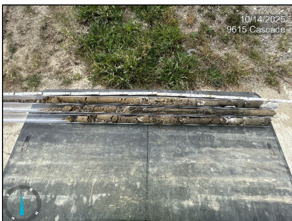
Photo 5: Viewing soil recovery from 9615 Cascade SB-1, SB-2, and SB-3
