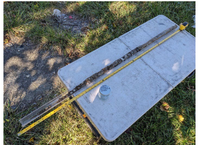
Photo 4. View of supplemental soil boring recovery
