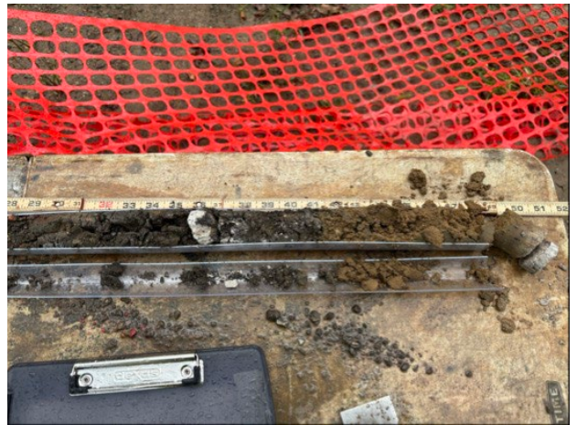
Photo 4. View of soil recovery at the time of TCLP soil boring activities
