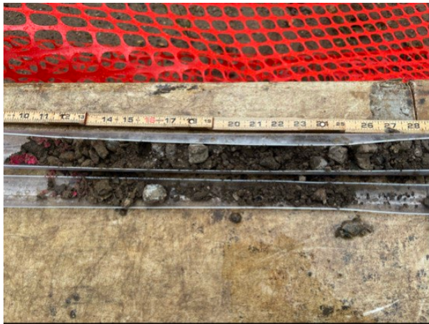
Photo 3. View of soil recovery at the time of TCLP soil boring activities
