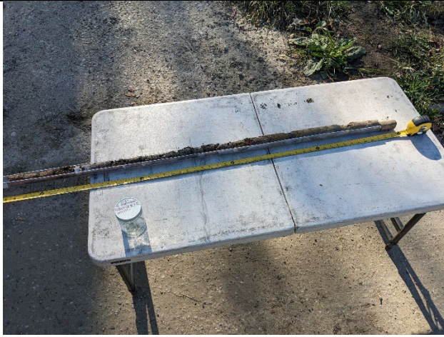
Photo 7. View of soil recovery at the time of supplemental soil sampling activities
