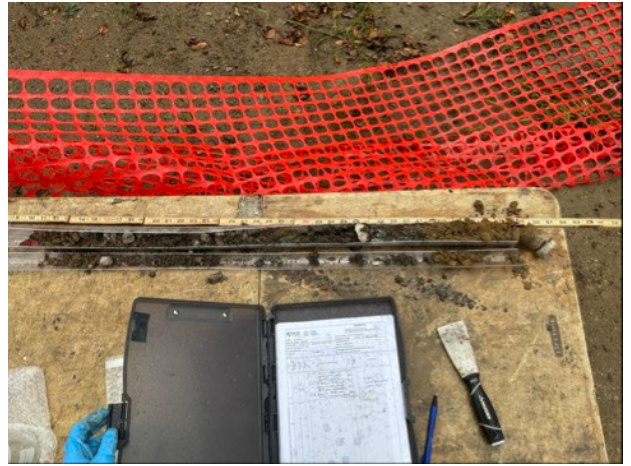
Photo 2. View of soil recovery at the time of TCLP soil boring activities
