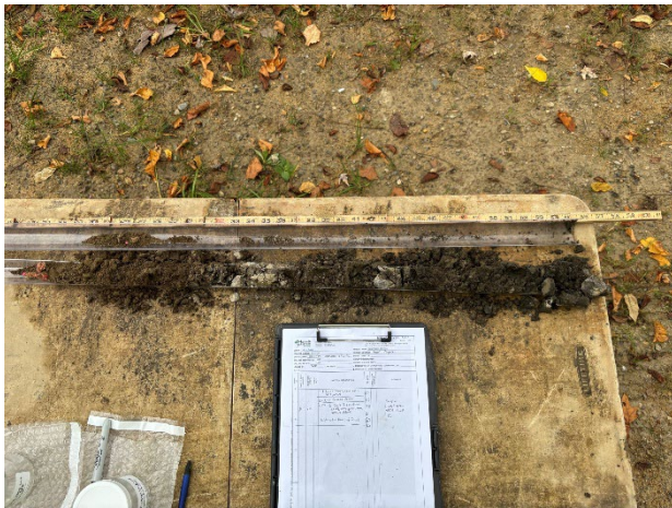
Photo 3. View of TCLP soil boring recovery
