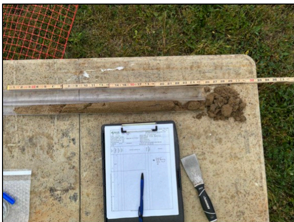
Photo 5: View of soil recovery at the time of TCLP sampling
