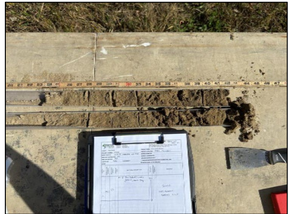
Photo 4: View of soil recovery at the time of TCLP sampling.
