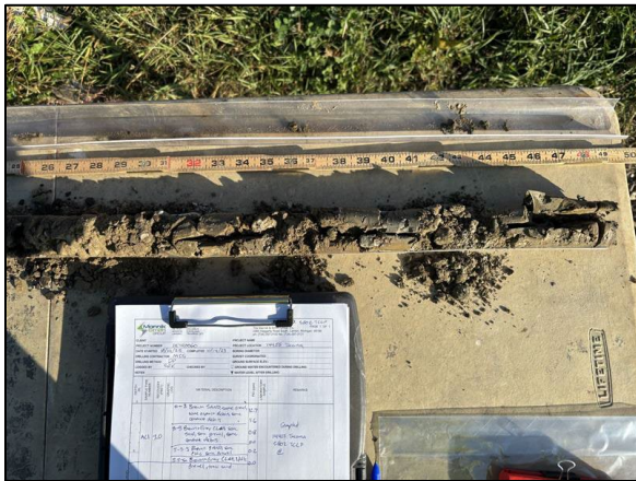
Photo 1: View of soil recovery at the time of TCLP sampling
